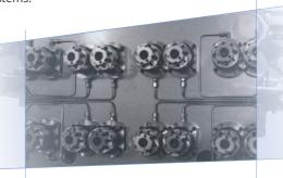
The workpieces reference and clamping fixture are all automatic with hydraulic or pneumatic command. Several parts machined in the same station to increase volume of production.
