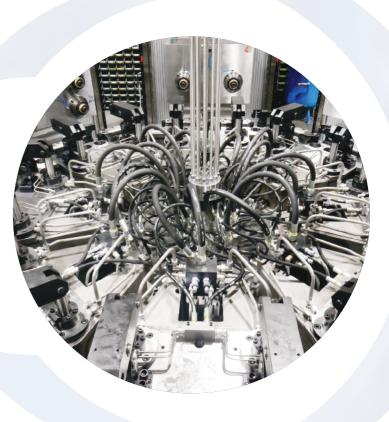
OTED - One touch exchange of dies exchange of dies to make transfers flexible
