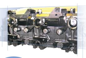
**The working** units are all with three-axis CNC controlled. The multi-spindle heads are designed for the optimal machining of the specific part and can have, even on the same structure, horizontal and vertical or tilted spindles.
